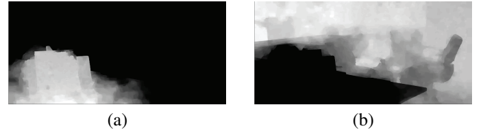
Fig. 8. (a) Negative disparity map d_{\text{map}}^- , where brighter regions are in front of the screen. (b) Positive disparity map d_{\text{map}}^+ where brighter regions are behind the screen.
