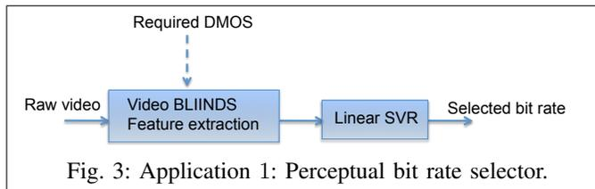
Fig. 3: Application 1: Perceptual bit rate selector.
