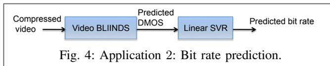
Fig. 4: Application 2: Bit rate prediction.
