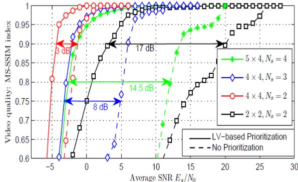
Fig. 4. Comparison of the loss visibility-based prioritization vs. non-prioritized MIMO precoding.
