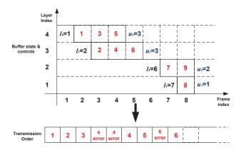
**Fig. 1**. Receiver buffer state, control and corresponding transmission order.
