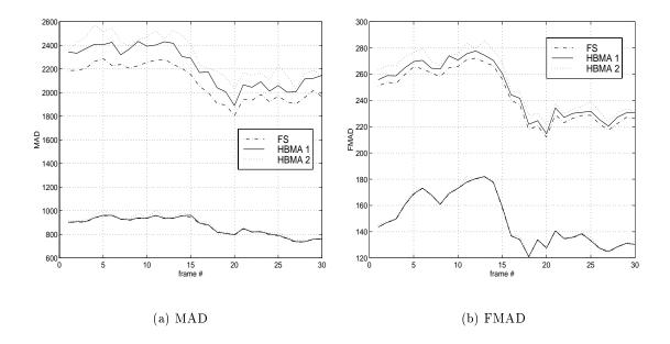
Fig. 7. The MAD (a) and the FMAD (b) of motion compensated frames according to "Mobile" frames. The 3 upper lines are for the regular video and the 3 lower lines are for the foveated video.
