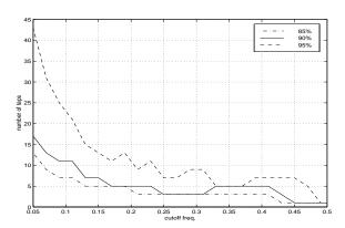
Fig. 4. The number of filter taps according to cutoff frequency
