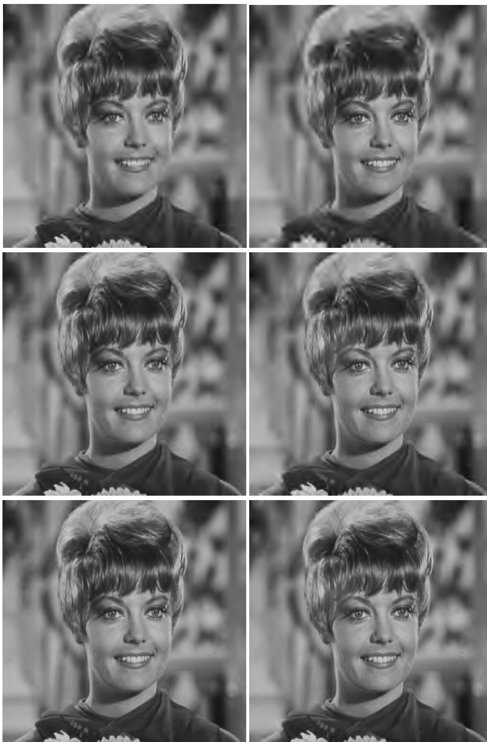
Fig.4 “Zelda” image compression result comparison. Top: Original image with the foveated ROI indicated; The left images that followed: SPIHT coded images; The right images that followed: EFIC coded images. The bit rates from top to bottom are 0.015625bpp (CR=512:1), 0.03125bpp (CR=256:1), 0.0625bpp (CR=128:1), 0.125bpp (CR=64:1), and 0.25bpp (CR=32:1), respectively.
