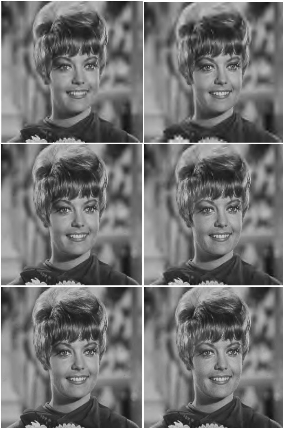
Fig. 13 “Zelda” image compression results. Top-left: Original image with the foveation region indicated; Top-right: DWT domain importance weighting mask for EFIC (Brightness logarithmically enhanced for display purpose); The images of the left column that follow: SPIHT coded images; The images of the right column that
